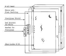
20" x 30" x 1/8 Seamed Edge Mirror with Foam Backing 20" x 30" x 3/32 Plexiglass Shield ■FRONT BEZEL (picture frame cover)
